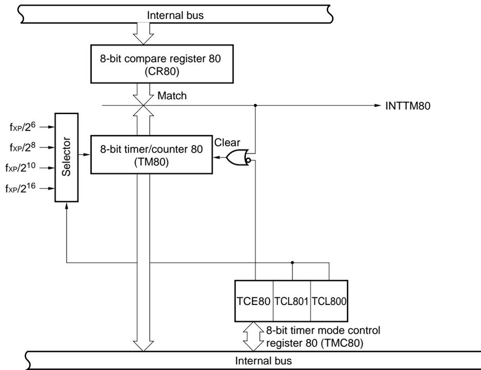
**Remark**  $f_{XP}$ : Oscillation frequency of clock to peripheral hardware
