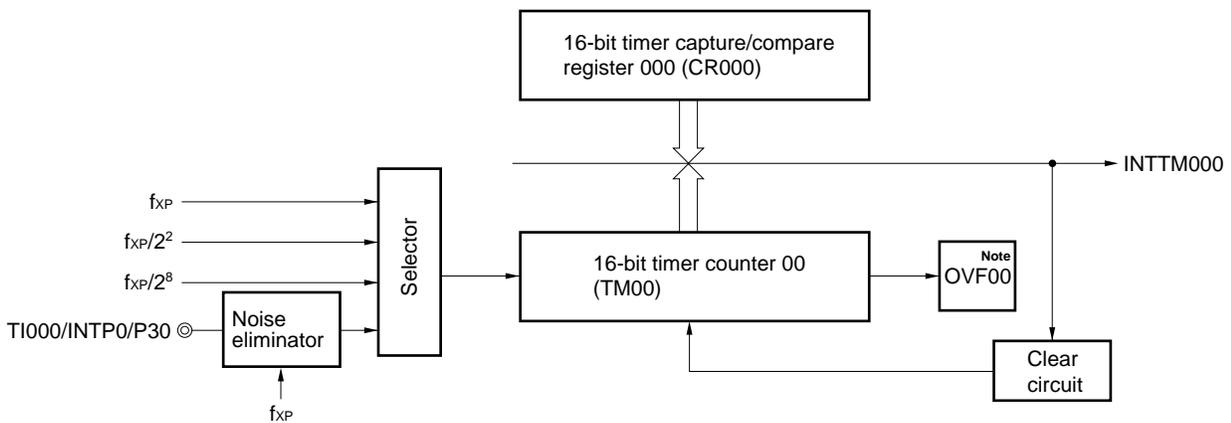
**Note** OVF00 is set to 1 only when 16-bit timer capture/compare register 000 is set to FFFFH.
