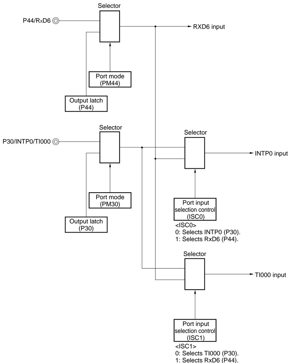
**Remark** ISC0, ISC1: Bits 0 and 1 of the input switch control register (ISC) (see **Figure 11-11**)
