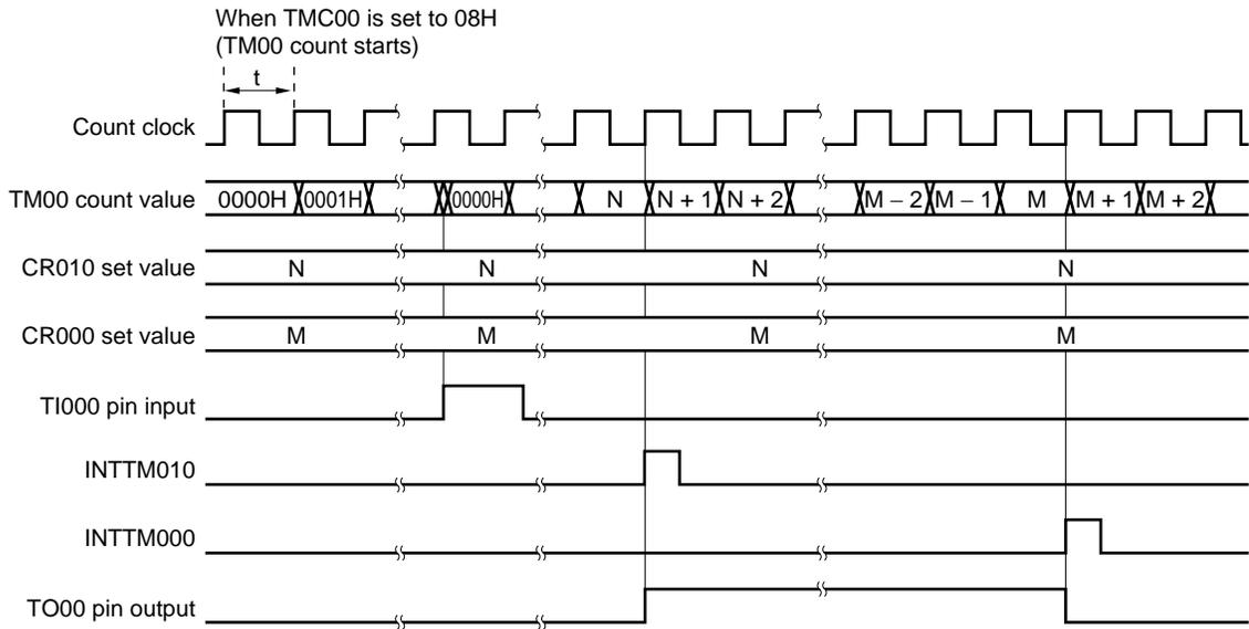
**Caution** 16-bit timer counter 00 starts operating as soon as a value other than 00 (operation stop mode) is set to the TMC002 and TMC003 bits.
