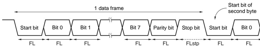
Where the 1-bit data length is  $FL$ , the stop bit length is  $FL_{stp}$ , and base clock frequency is  $f_{CLK6}$ , the following expression is satisfied.
