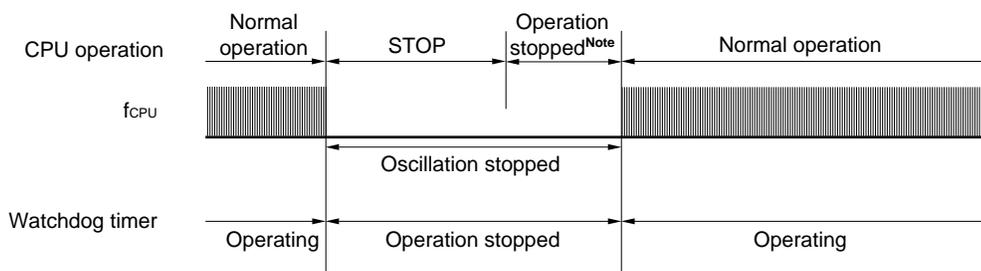
**Note** The operation stop time is 17  $\mu$ s (MIN.), 34  $\mu$ s (TYP.), and 67  $\mu$ s (MAX.).
