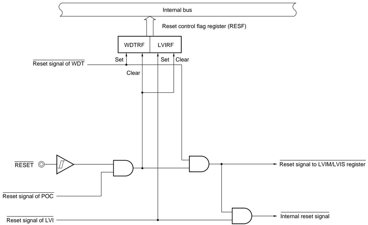
**Caution** The LVI circuit is not reset by the internal reset signal of the LVI circuit.
