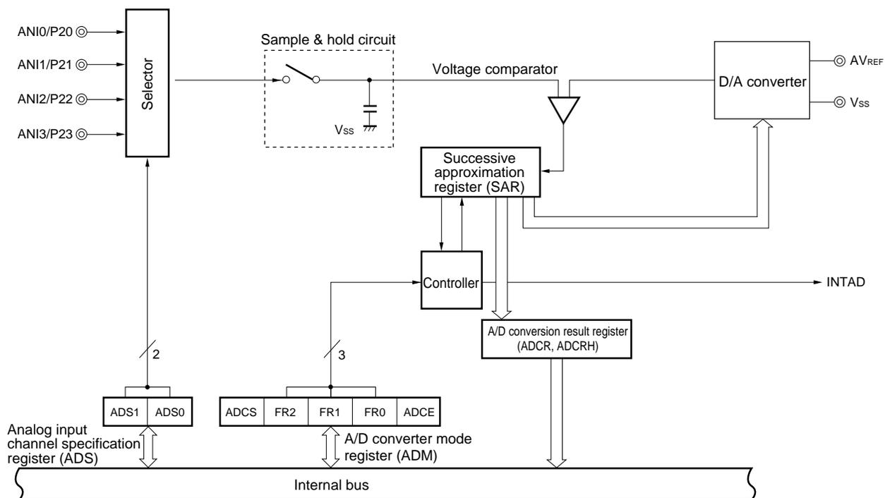
**Caution** In the 78K0S/KA1+,  $V_{SS}$  functions alternately as the ground potential of the A/D converter. Be sure to connect  $V_{SS}$  to a stabilized GND (= 0 V).
