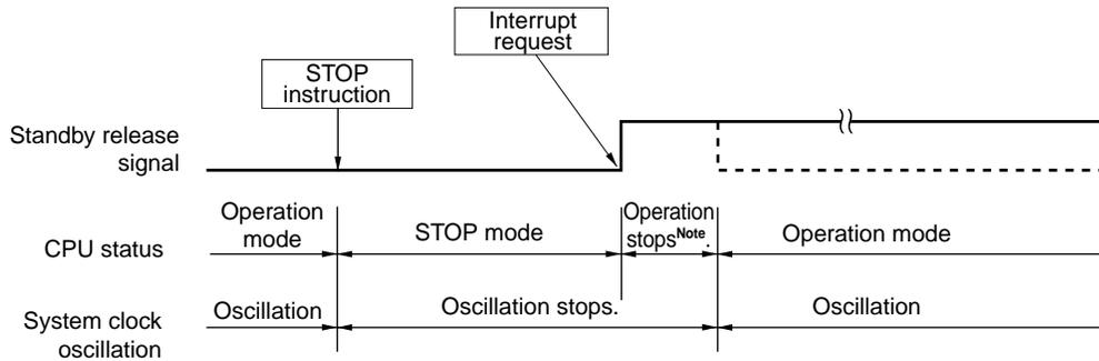
(2) If CPU clock is crystal/ceramic oscillation clock
