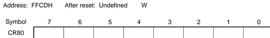
**Caution** When changing the value of CR80, be sure to stop the timer operation. If the value of CR80 is changed with the timer operation enabled, a match interrupt request signal is generated immediately and the timer may be cleared.
