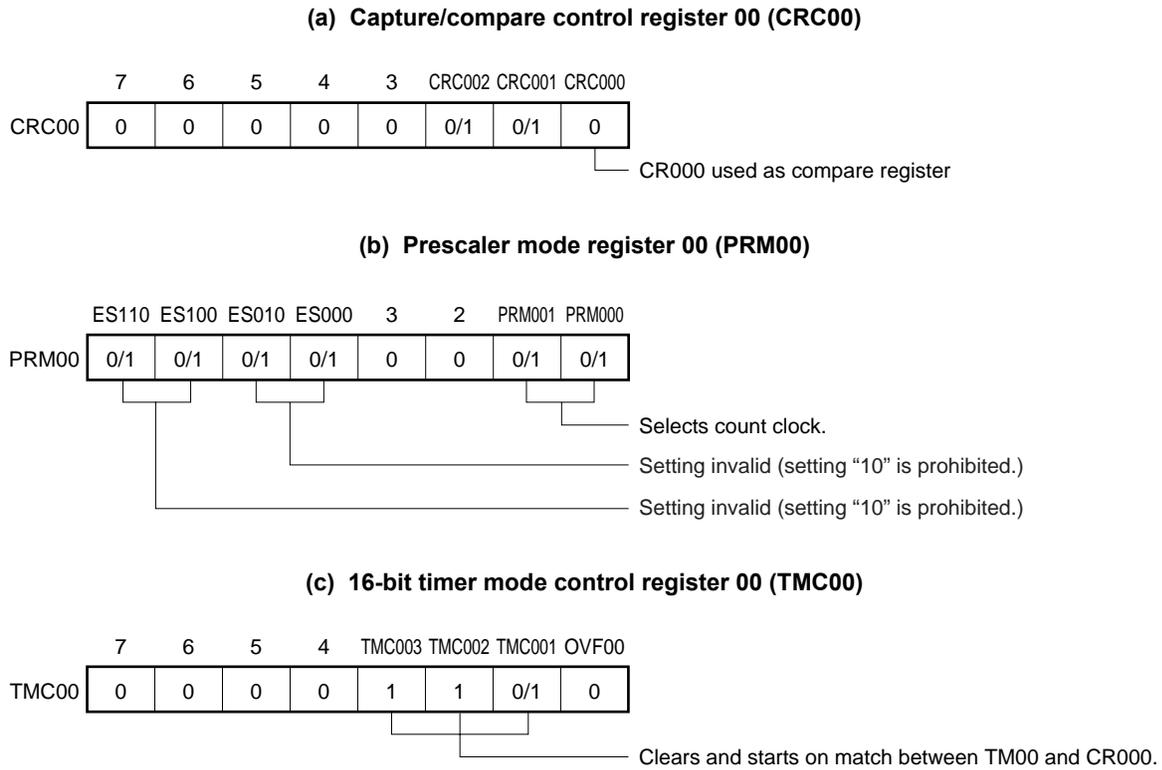
**Remark** 0/1: Setting 0 or 1 allows another function to be used simultaneously with the interval timer. See the description of the respective control registers for details.
