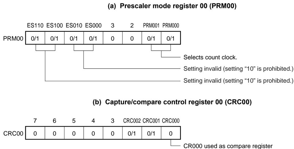
Figure 6-27. Control Register Settings in Square-Wave Output Mode (2/2)
