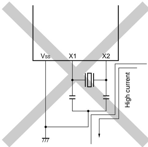
(d) Current flowing through ground line of oscillator
