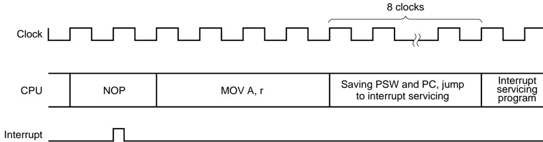
If an interrupt request flag ( $\times\times$ IF) is set at the last clock of the instruction, the interrupt acknowledgment processing starts after the next instruction is executed.
