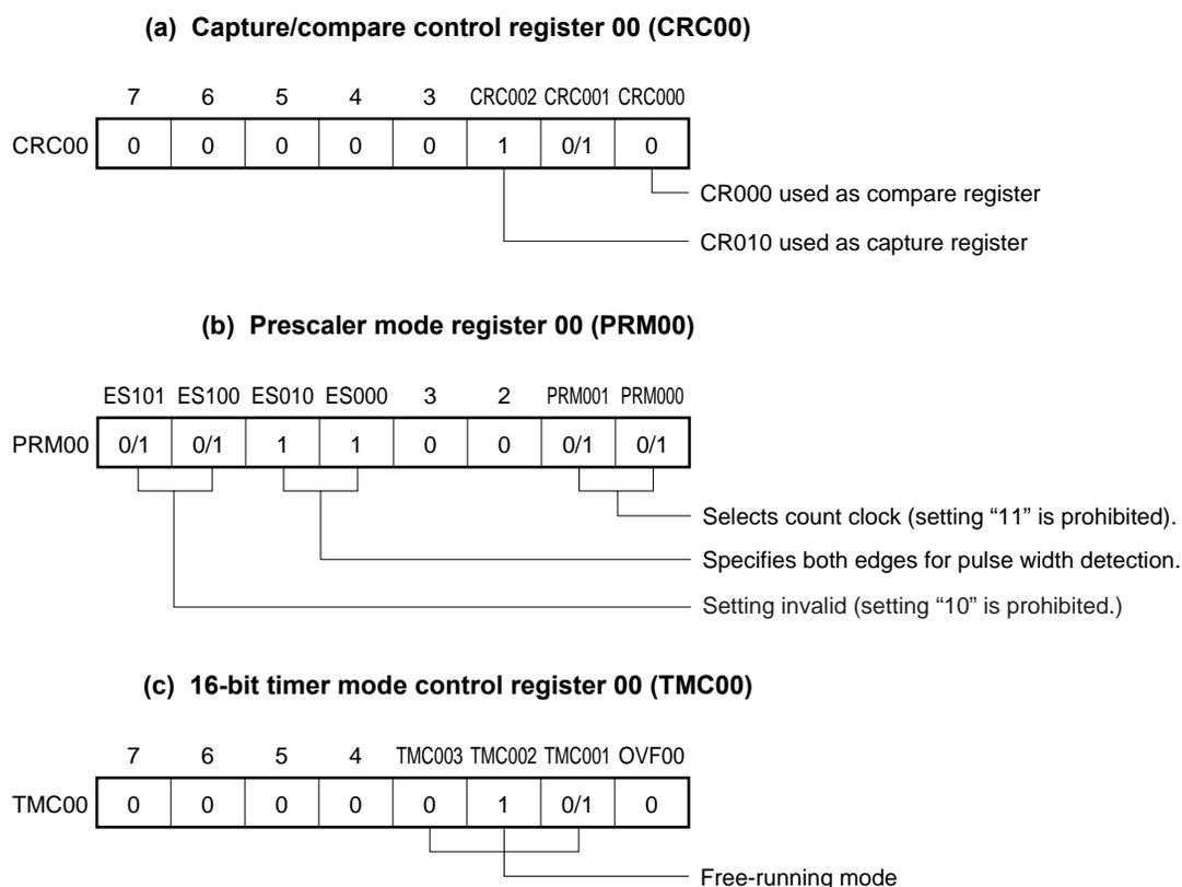
**Remark** 0/1: Setting 0 or 1 allows another function to be used simultaneously with pulse width measurement. See the description of the respective control registers for details.
