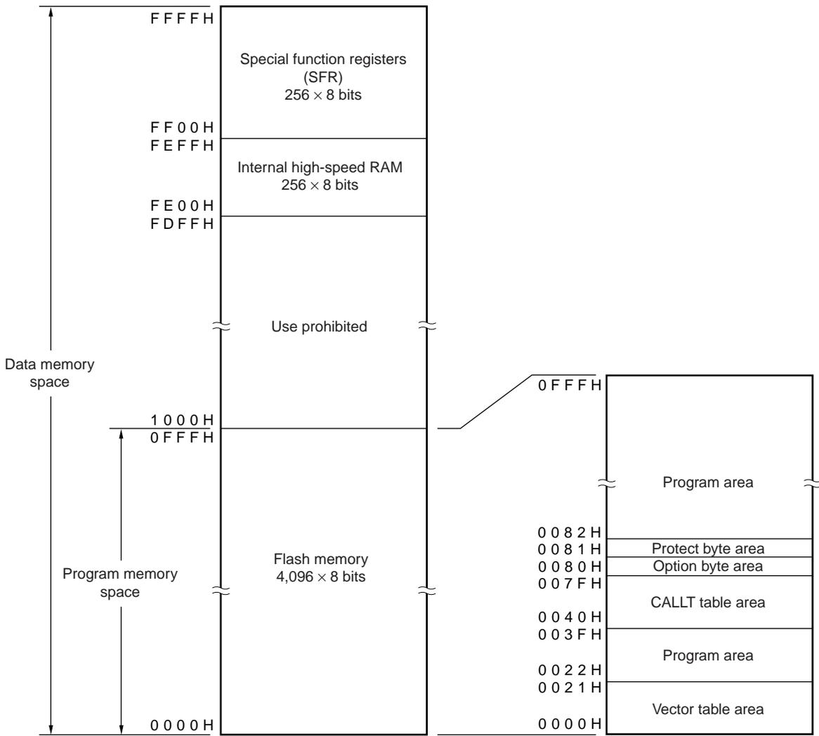
**Remark** The option byte and protect byte are 1 byte each.
