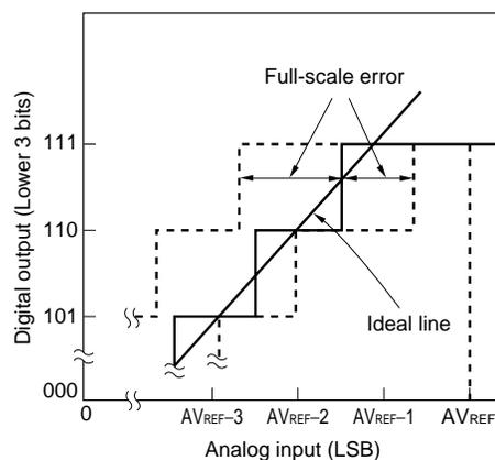
**Figure 10-17. Integral Linearity Error**
