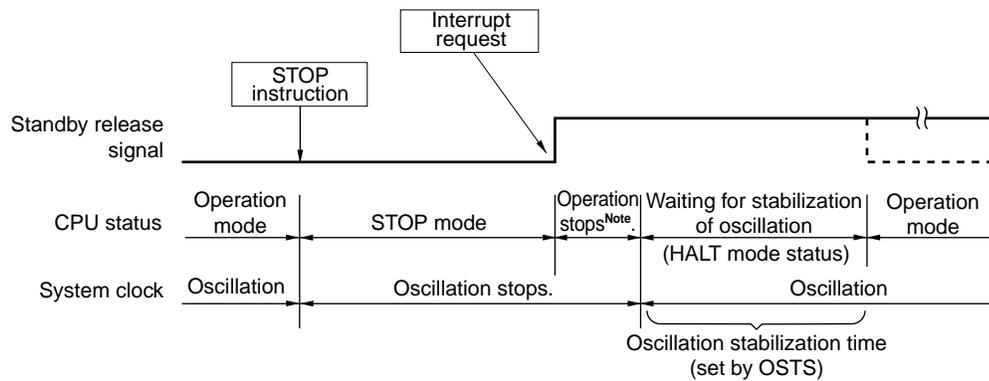
**Note** The operation stop time is 17  $\mu\text{s}$  (MIN.), 34  $\mu\text{s}$  (TYP.), and 67  $\mu\text{s}$  (MAX.).
