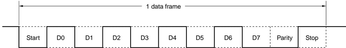
2. Data length: 8 bits, MSB first, Parity: Even parity, Stop bit: 1 bit, Communication data: 55H
