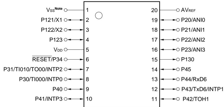
**Note** In the 78K0S/KA1+, V<sub>ss</sub> functions alternately as the ground potential of the A/D converter. Be sure to connect V<sub>ss</sub> to a stabilized GND (= 0 V).
