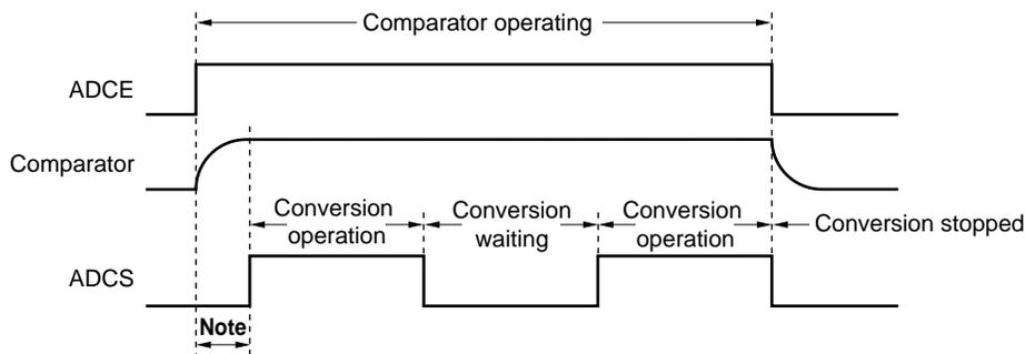
**Note** The time from the rising of the ADCE bit to the rising of the ADCS bit must be  $1\ \mu\text{s}$  or longer to stabilize the internal circuit.
