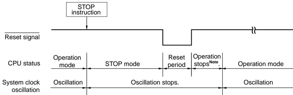
**Note** Operation is stopped (277  $\mu$ s (MIN.), 544  $\mu$ s (TYP.), 1.075 ms (MAX.)) because the option byte is referenced.
