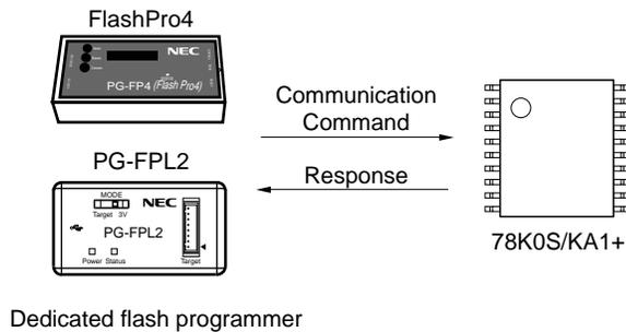
Communication commands are listed in the table below. All these communication commands are issued from the programmer and the 78K0S/KA1+ perform processing corresponding to the respective communication commands.
