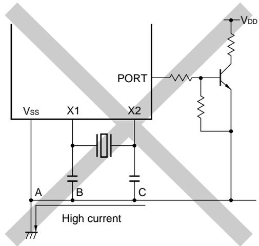
Figure 5-7. Examples of Incorrect Resonator Connection (2/2)
