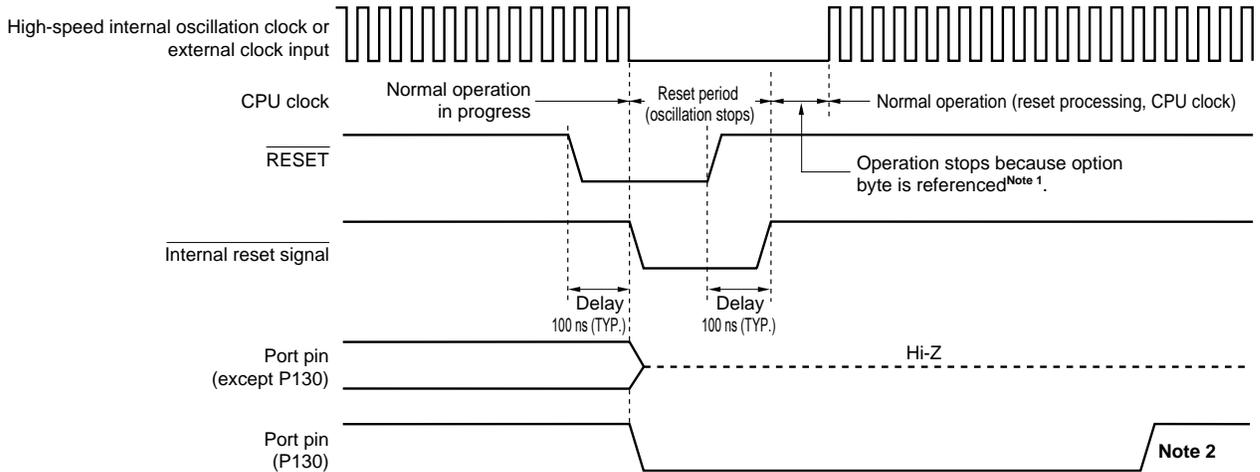
**Notes 1.** The operation stop time is 277  $\mu\text{s}$  (MIN.), 544  $\mu\text{s}$  (TYP.), and 1.075 ms (MAX.).
