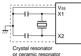
**Caution** When using the crystal/ceramic oscillator, wire as follows in the area enclosed by the broken lines in Figure 5-6 to avoid an adverse effect from wiring capacitance.
