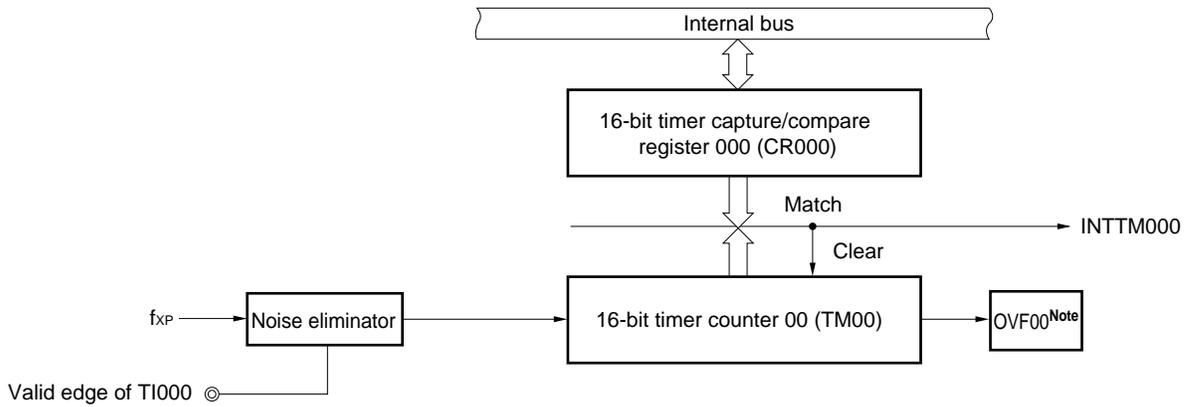
**Note** OVF00 is 1 only when 16-bit timer capture/compare register 000 is set to FFFFH.
