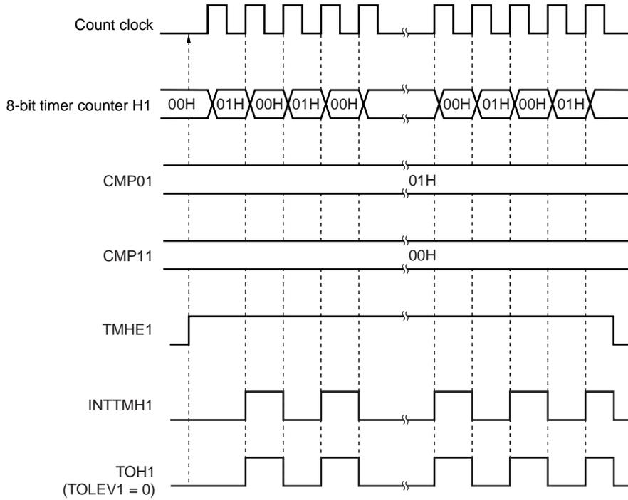
Figure 8-9. Operation Timing in PWM Output Mode (4/4)
