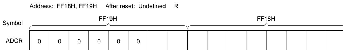
**Caution** When writing to the A/D converter mode register (ADM) and analog input channel specification register (ADS), the contents of ADCR may become undefined. Read the conversion result following conversion completion before writing to ADM and ADS. Using timing other than the above may cause an incorrect conversion result to be read.
