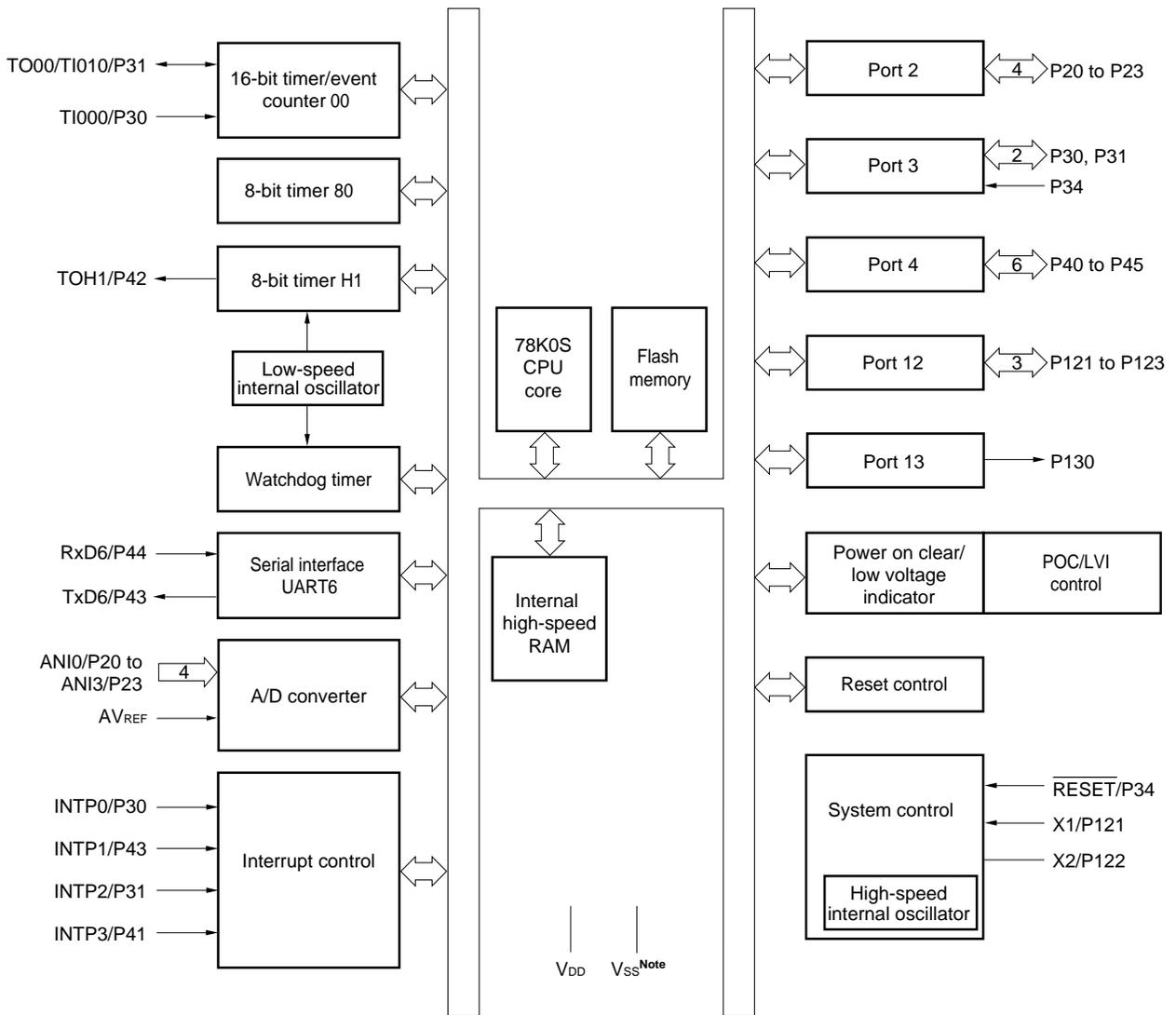
**Note** In the 78K0S/KA1+,  $V_{SS}$  functions alternately as the ground potential of the A/D converter. Be sure to connect  $V_{SS}$  to a stabilized GND (= 0 V).
