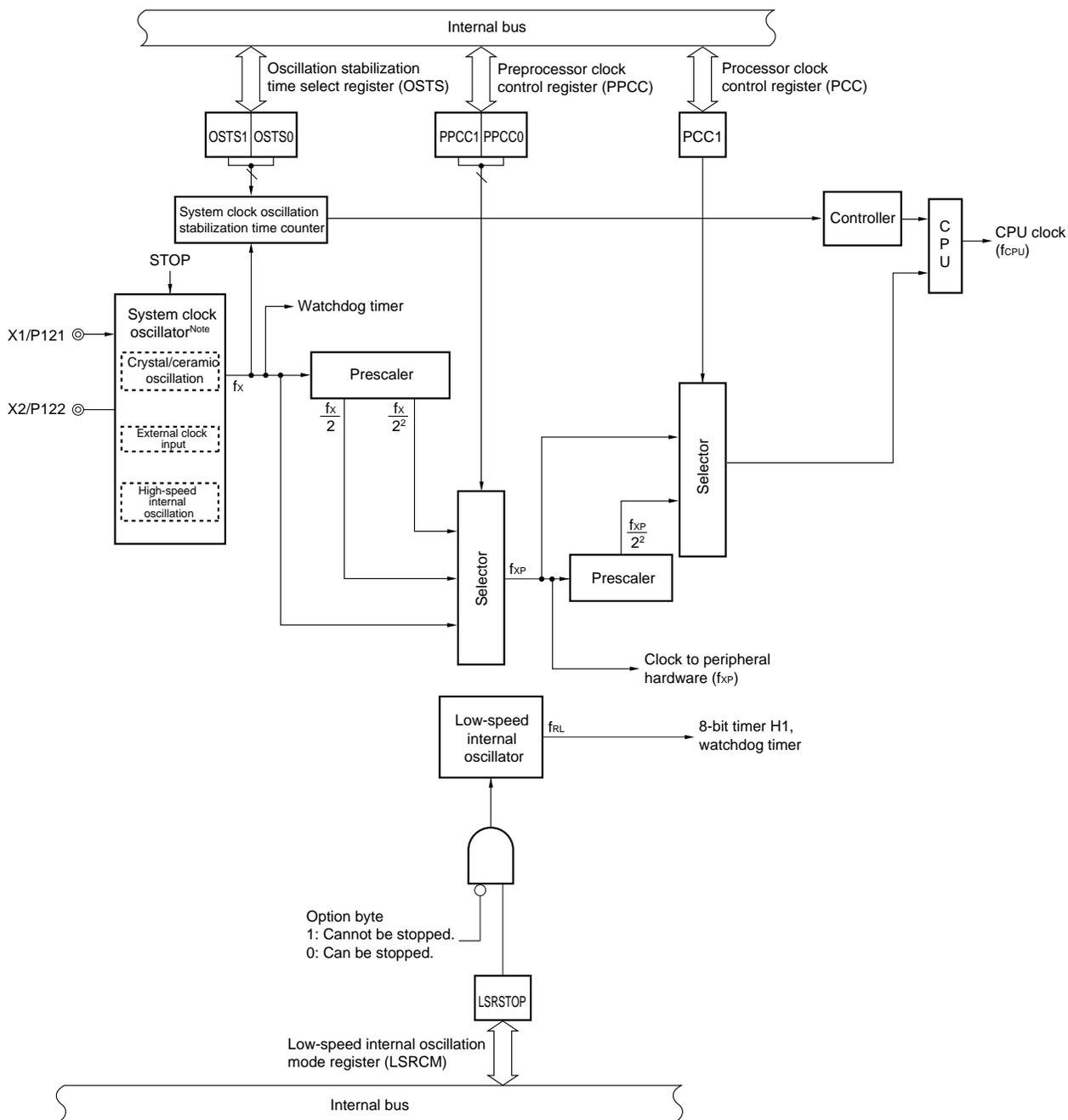
**Note** Select the high-speed internal oscillator, crystal/ceramic oscillator, or external clock input circuit as the system clock source by using the option byte.
