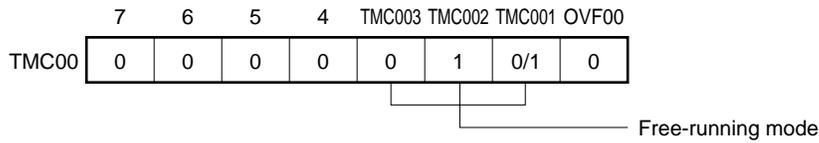
**Remark** 0/1: Setting 0 or 1 allows another function to be used simultaneously with pulse width measurement. See the description of the respective control registers for details.
