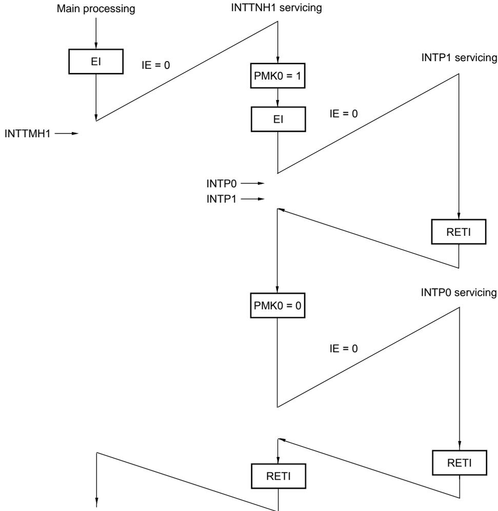
In the interrupt INTTMH1 servicing, servicing is performed such that the INTP1 interrupt is given priority, since the INTP0 interrupt was first masked.
