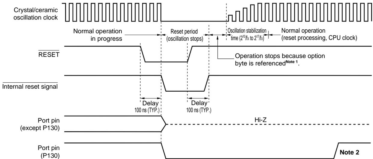
**Notes 1.** The operation stop time is 276  $\mu\text{s}$  (MIN.), 544  $\mu\text{s}$  (TYP.), and 1.074 ms (MAX.).
