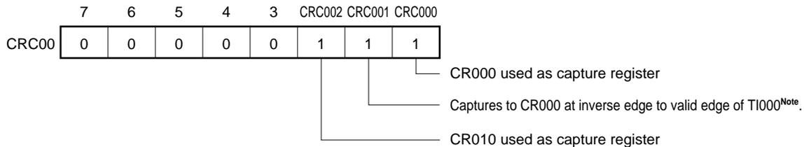
**Figure 6-25. Control Register Settings for Pulse Width Measurement by Means of Restart (with Rising Edge Specified) (2/2)**
