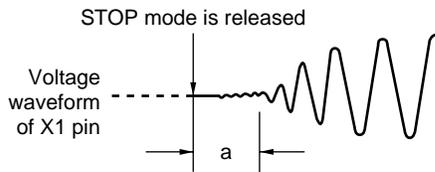
3. The oscillation stabilization time that elapses on power application or after release of reset is selected by the option byte. For details, refer to **CHAPTER 17 OPTION BYTE**.
