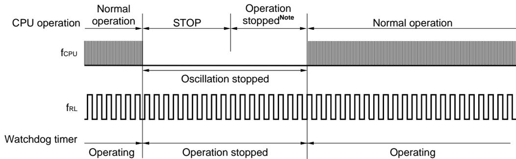
**Note** The operation stop time is 17  $\mu s$  (MIN.), 34  $\mu s$  (TYP.), and 67  $\mu s$  (MAX.).
