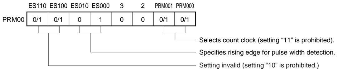
**(c) 16-bit timer mode control register 00 (TMC00)**
