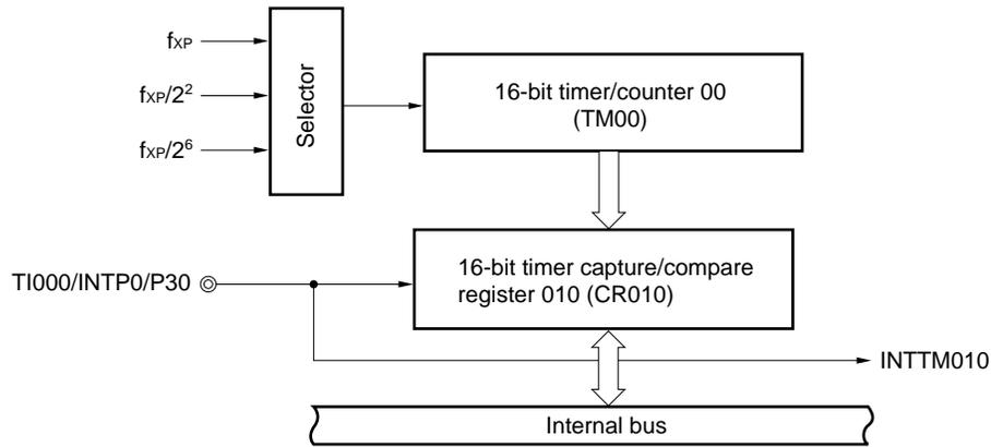
★ **Figure 6-20. Timing of Pulse Width Measurement Operation by Free-Running Counter and One Capture Register (with Both Edges Specified)**
