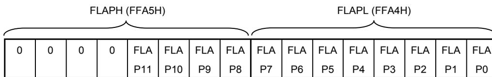
★ **Caution** Be sure to clear bits 4 to 7 of flash address pointer H (FLAPH) and flash address pointer H compare register (FLAPHC) to 0 before executing the self programming command. If the value of these bits is 1 when executing the self programming command.
