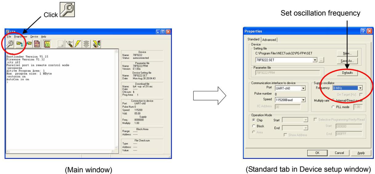
Table 18-5. Oscillation Frequency and PG-FP4 GUI Software Setting Value Example
