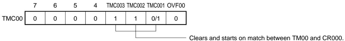
**Remark** 0/1: Setting 0 or 1 allows another function to be used simultaneously with the external event counter. See the description of the respective control registers for details.
