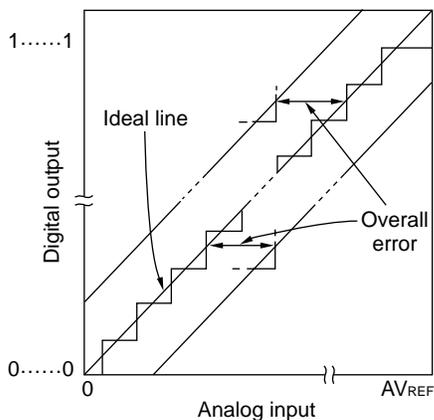
Figure 10-14. Quantization Error
