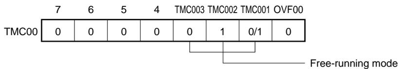
★ **Note** If the valid edge of TI000 pin is specified to be both the rising and falling edges, 16-bit timer capture/compare register 000 (CR000) cannot perform the capture operation. When the CRC001 bit value is 1, the TM00 count value is not captured in the CR000 register when a valid edge of the TI010 pin is detected, but the input from the TI010 pin can be used as an external interrupt source because INTTM000 is generated at that timing.
