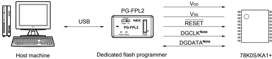
★ **Note** DGCLK is a clock for communication, while DGDATA is a transmit/receive signal for communication data.
