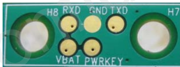
Figure 13: Upgrade test points
