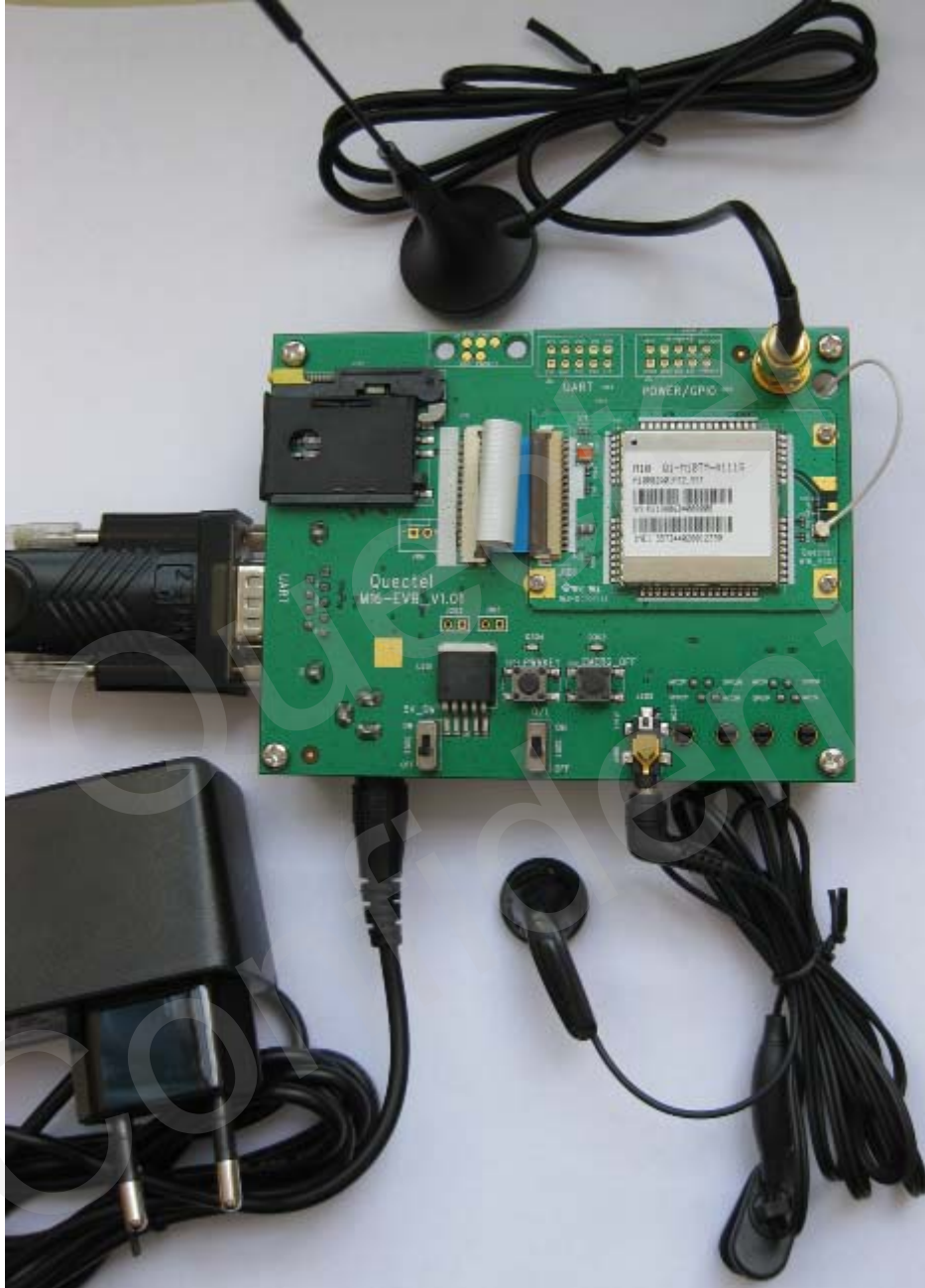
Figure 14: Assembled EVB and accessories
