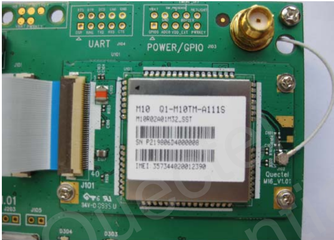
Figure 17: Fix module and RF cable
