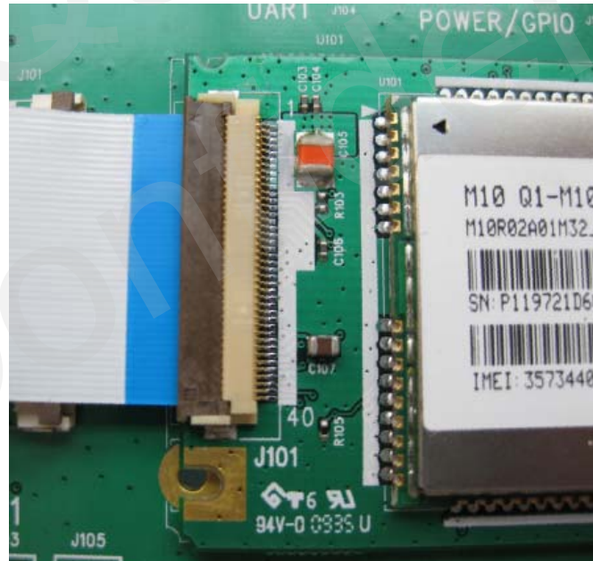
Figure 16: FPC connected to ZIF connector of module
