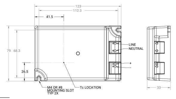
1 Dimensions for all the LMD125 diagrams are in mm and are for reference only. For exact dimensions and tolerances, refer to the 3-D models (.STEP files) for the LMD125 drivers available by selecting the Documentation tab on the LMH2 product page.
