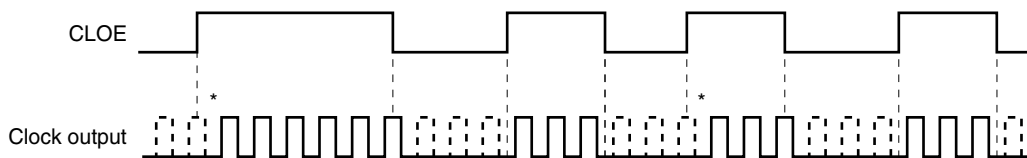
Figure 11-4. Remote Control Output Application Example
