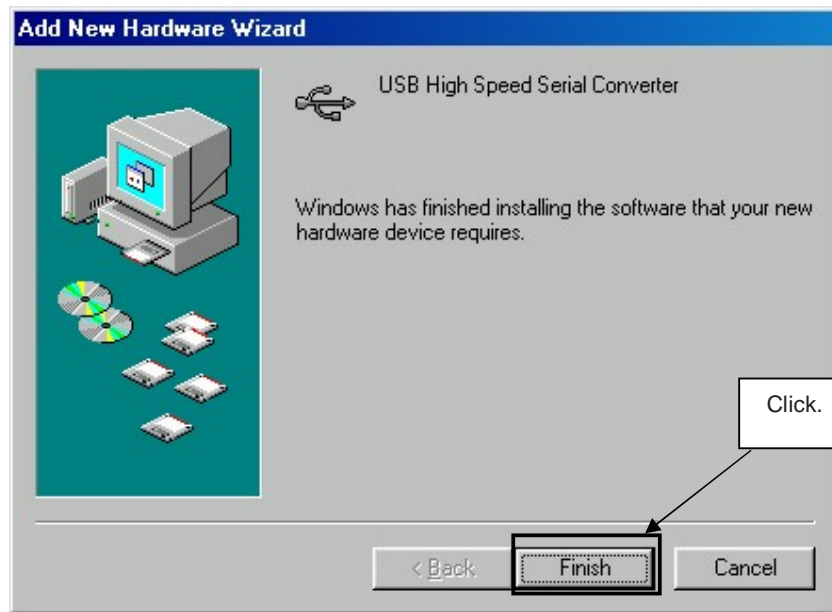
Figure 14: Installation Completion (Windows 98SE)
