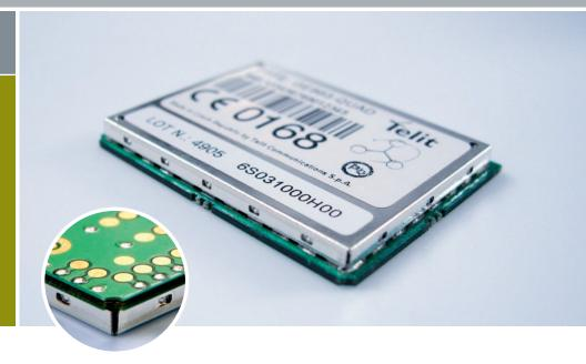
The GE863-QUAD module is now boasting quad-band functionality and RoHS compliance and additional new features. This translates into one consistent product offering for global GSM networks and provides for significant cost advantages with the savings in approvals and logistics costs.
