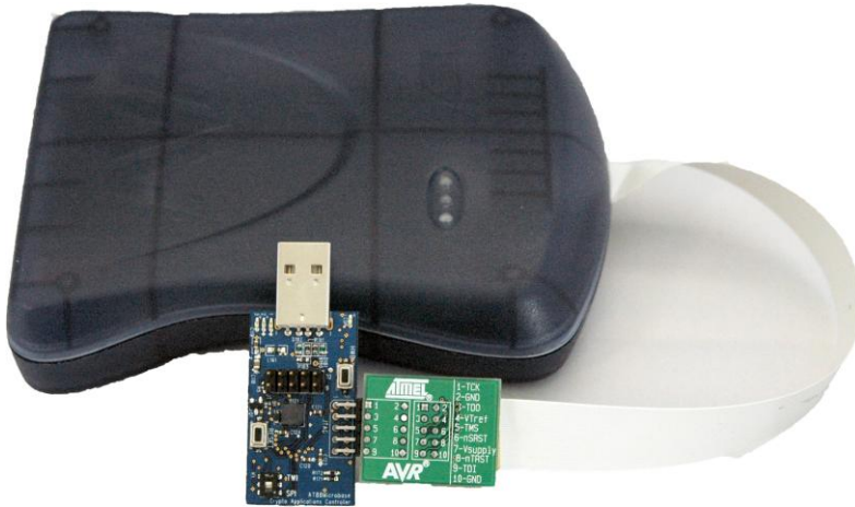
Figure 1-11. Connecting the Atmel AVR JTAGICE mkII to the Atmel AT88Microbase
