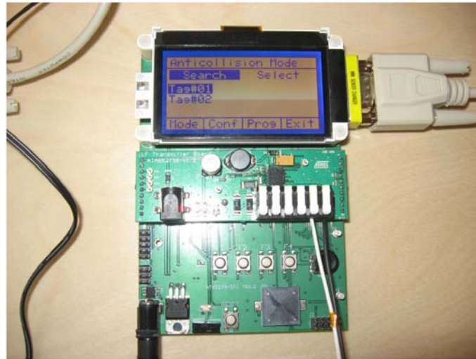
Figure 5-3. Anticollision Mode Device Search Results
