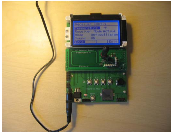
Figure 3-2. The RF Receiver Board Configuration Menu
