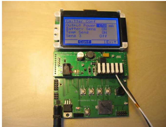
Figure 2-3. LF Driver Board Configuration Menu (E.G., Setting Output Power to 650mA)
