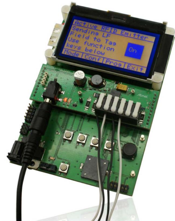
Figure 2-2. LF Driver Top-Level LCD Menu
