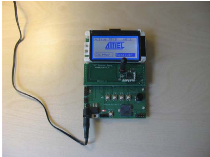
Figure 3-1. RF Receiver Board Assembly
